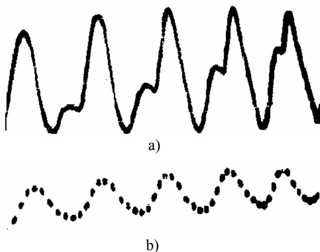
Fig. 2. low-frequency photocurrent oscillations ( $\sim 2$  Hz) at different intensity of a light:  $I_a < I_b$  (of quantum energy -  $h\nu \geq 0.9$  eV, Intensity of an electric field - 50 V/cm)
