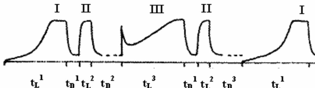
Fig. 1. Typical photocurrent kinetics of GaAs irradiated with accelerated electrons at different annealing stages
