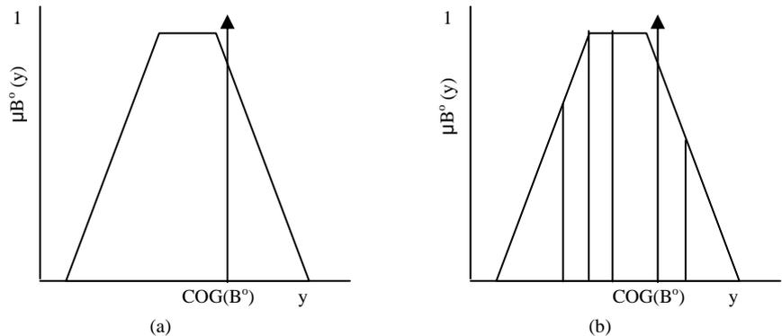
Figure 2.2: COG defuzzification method (a) Continuous (b) Discrete
