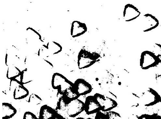
Fig.1. Dislocation structure of SiGe alloy single crystal with 0.4at%Ge(x1000) on the plane[111]
