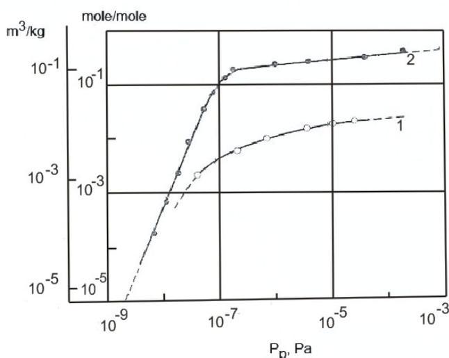
Fig.2. Isotherms of adsorption of He (curve 1) and  $H_2$  (curve 2) on Ar condensate  $\sim 10^{-4}$  monolayer thick at  $T=4.2$ K.
