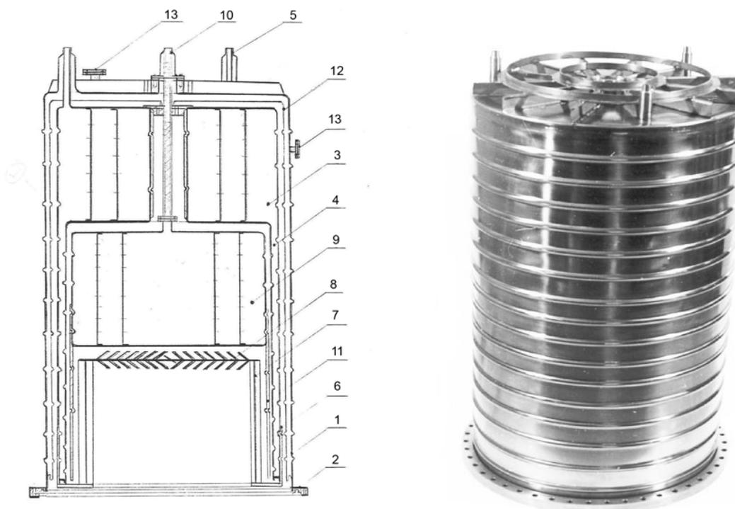
Fig.1. Section of a general view of the CCP-8D cryocondensation pump with the enveloped pumping zone.
