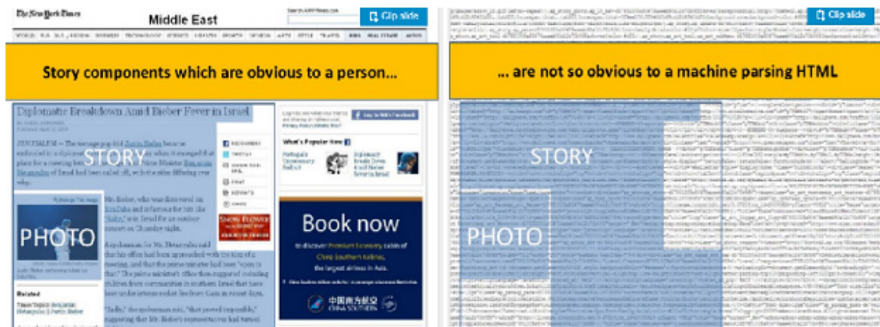
Figure 1. Differences between human reception and machine parsing HTML of websites (from official IPTC website)
