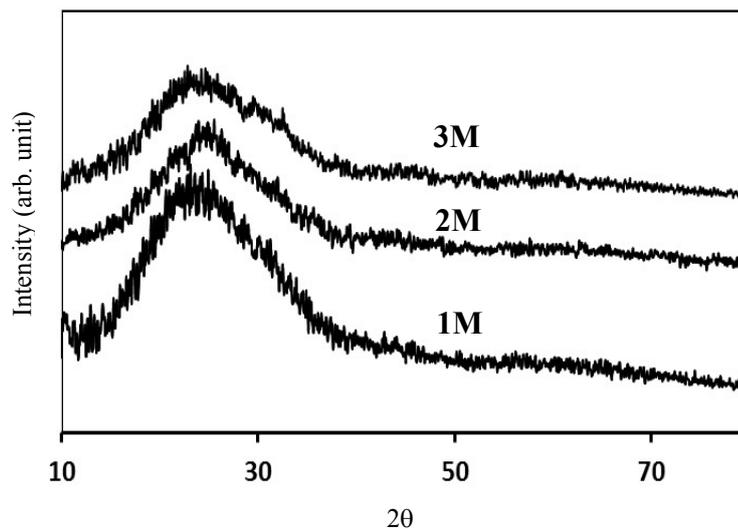
Fig. 1 The XRD spectra of PANI/TiO<sub>2</sub> nanocomposite thin films at different HCl molarity.
