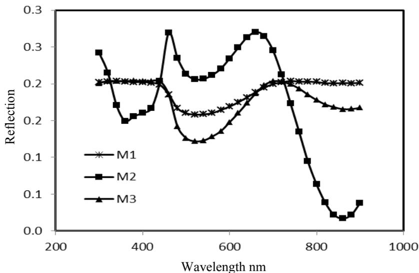
Fig. 3 reflectance spectra of PANI/TiO<sub>2</sub> nanocomposite thin films.
