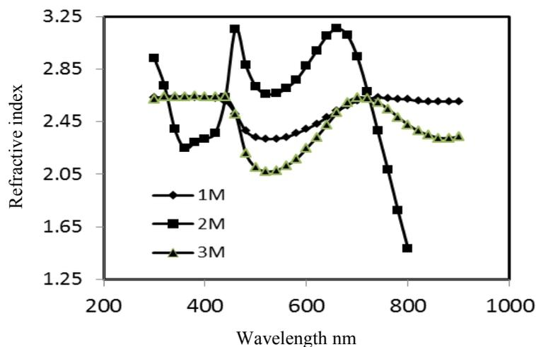
Fig. 6 The refractive index of PANI/TiO<sub>2</sub> nanocomposite thin films.
