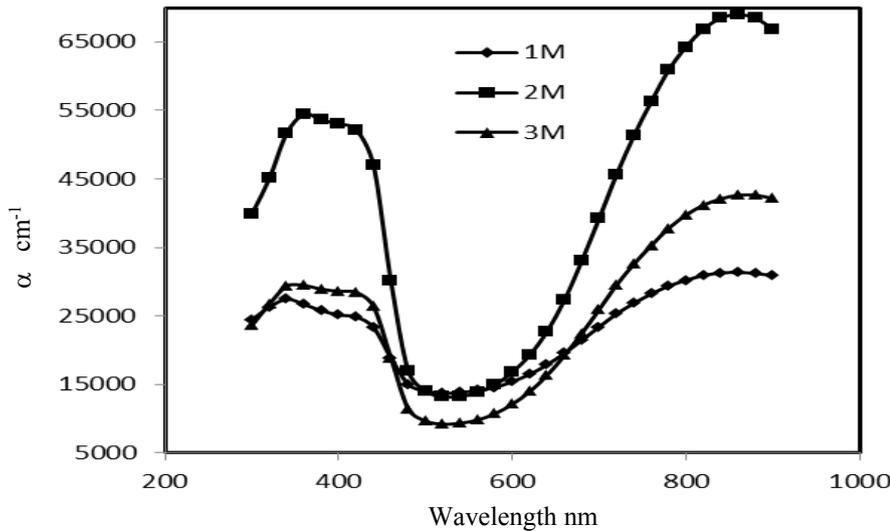
Fig. 4 The absorption coefficient of PANI/TiO<sub>2</sub> nanocomposite thin films.
