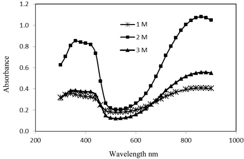
Fig. 2 Absorbance spectra of PANI/TiO<sub>2</sub> nanocomposite thin films.
