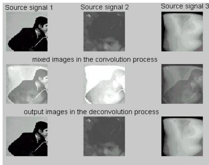
Figure 2: the source signals, the convolution signals and the deconvolution outputs
