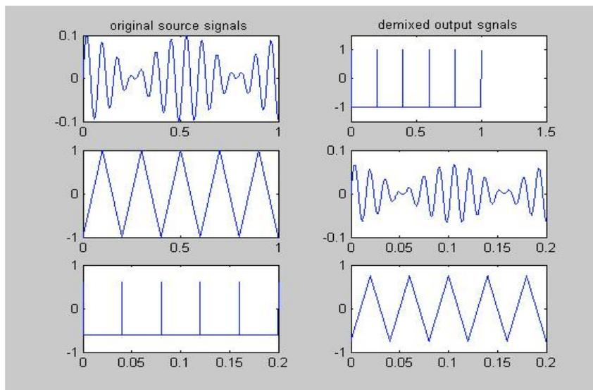
Figure (4) displays the waveforms of the source signals and the signals produced at the output of the demixer. It can be observed those after 3000 iterations; source signals are well separated
