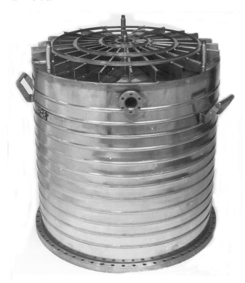
• Superhigh vacuum sorption pumps cooled by liquid nitrogen
