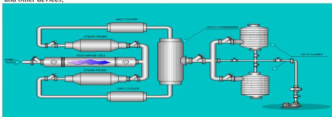
• Superhigh vacuum priming cryocondensing - sorption pumps cooled by liquid helium A range of their working pressure is from 10<sup>-3</sup> up to 10<sup>-11</sup> Pa. There have been developed and manufactured three various modifications with the pumping speed from 5.0 up to 10.0 m<sup>3</sup>/sec. One priming of liquid helium into the cryo-pump is enough for its continuous work from 2 to 4 months.
