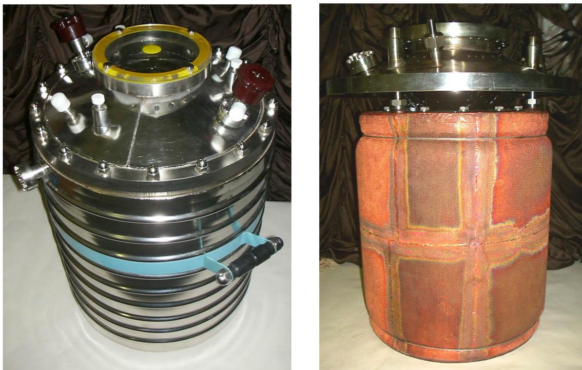
Fig.2 Cryosorption pump CSP-1.5D
