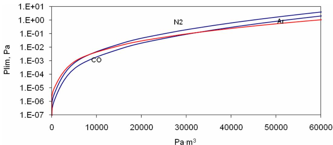
Fig.3. Dependence of limit pressure on amount of adsorbed gas
