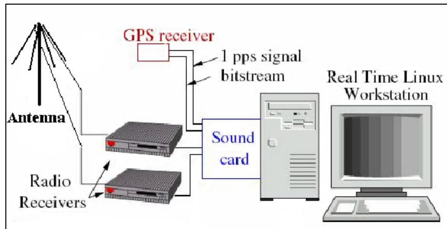
**Fig.10** Experimental setup for the Radio Detector System reception station
