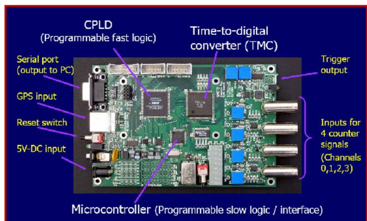
**Fig.2** Layout of DAQ Board (Qnet II) with major components labeled.
