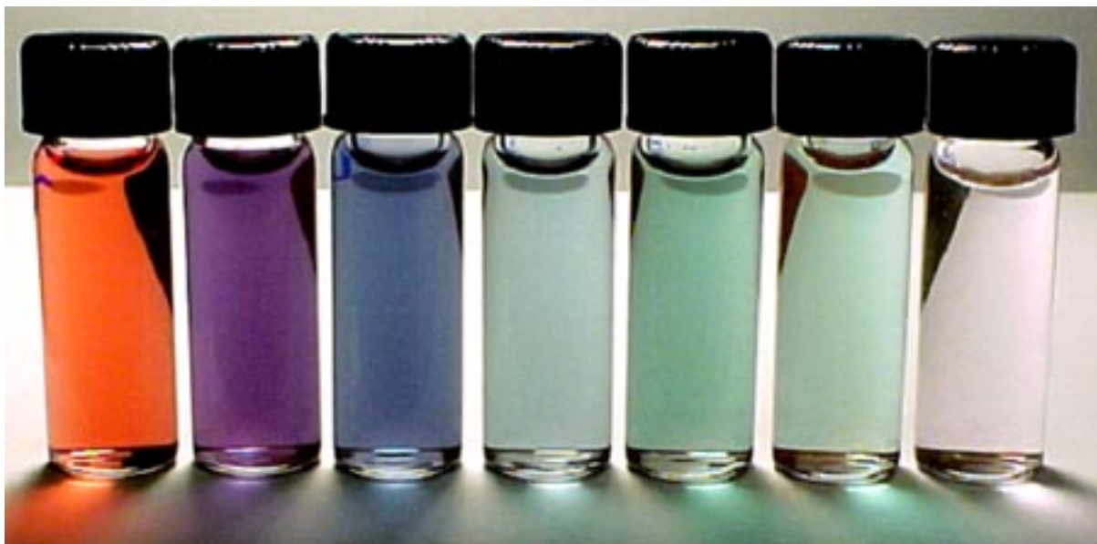
Figure 21: Nanoshells designed to absorb various wavelengths of light (the six vials on the right), including infrared (vial at far right) compared to gold colloid (far left). – nanospectra.com
