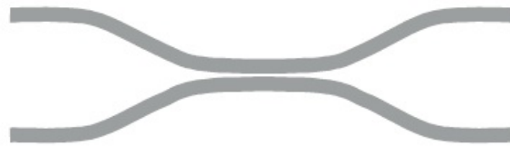
Figure 1 Waveguide structure consisting of two waveguides that are brought into close proximity over a finite distance. In the area where the two waveguides are close, the modes of the waveguides will interact, which means that their propagation vectors will be shifted, and their modes modified. Our starting point is the scalar wave equation:
