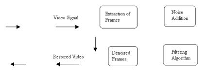
Fig. 3. Noise removal process
